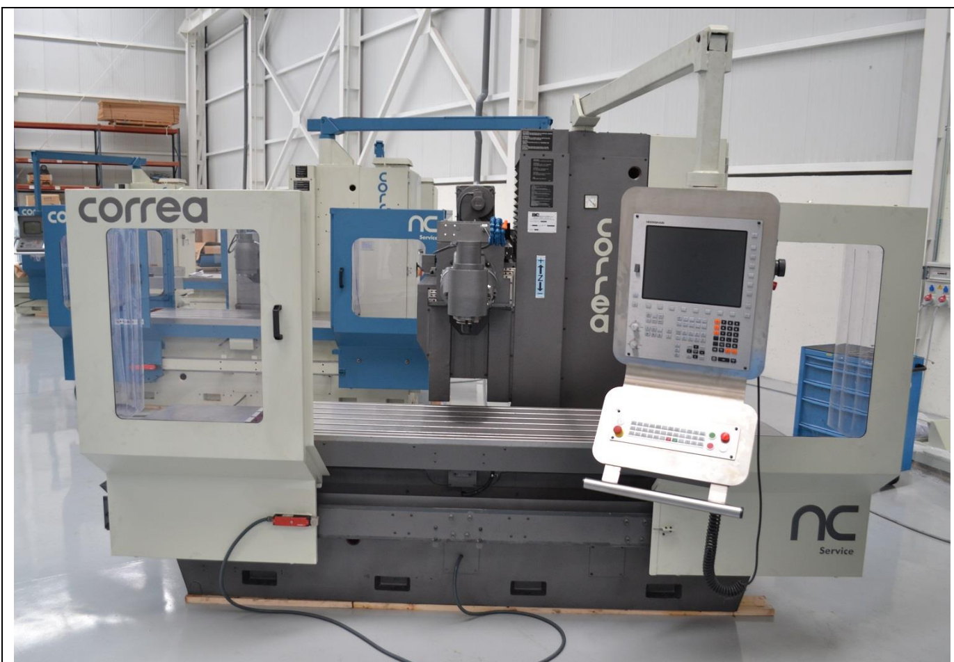
Milling bed type CORREA A16
