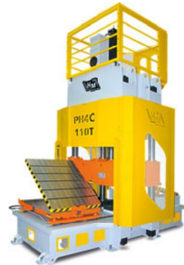
H-Frame Hydraulic Press equipped with ram guided by linear guides provides greater precision and there is a moveable lower table that slides on tracks with spheres and support braces. An articulating ram option with hydraulic locking, optional wax injection, guarantees the precision recommended for the adjustments of molds, dies, and tools. Pressing capacity up to 750 tons.
